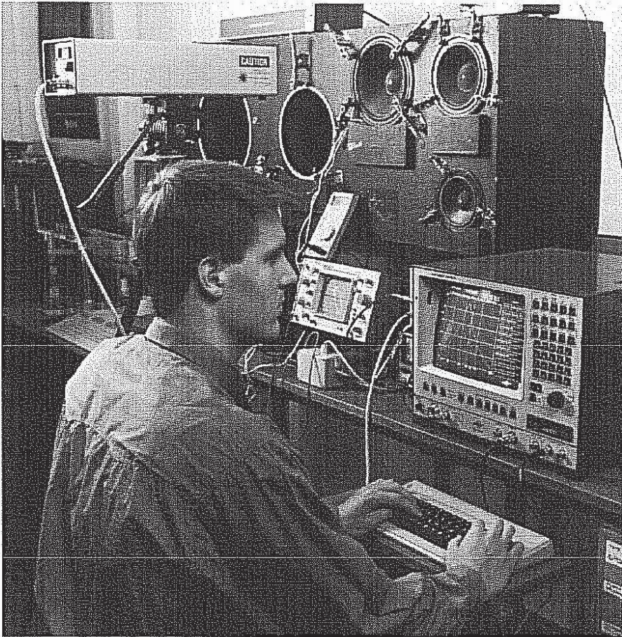
Fig. 13 Type 2012 is ideal for transducer measurements. The setup in the picture uses the Laser Transducer Set Type 3544 for measuring the Thiele-Small parameters. Use of the laser enables measurements without the mass-loading effects of an accelerometer
