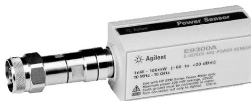
**Agilent E9300 sensors measure the average power of any signal format.**
