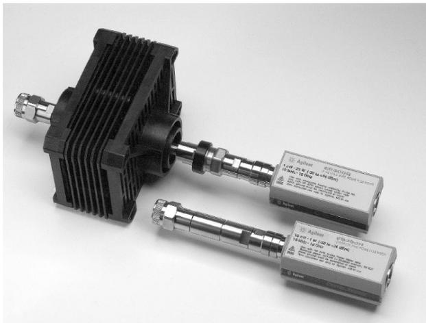
The Agilent Technologies E-series E9300 power sensors simplify your measurement equipment requirement and save you time and money, as well. Used with the Agilent E4418 (single-channel) and E4419 (dual-channel) EPM series power meters, these new sensors can measure the average power of RF and microwave signals, regardless of the modulation format, over a wide 80 dB dynamic range (sensor dependent).
