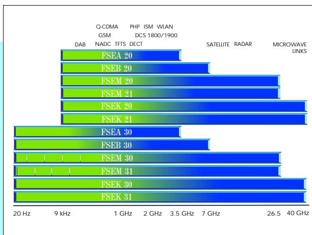
The vector signal analyzer option can be used with all analyzers of the FSE family to cover the frequency range up to 40 GHz for future-oriented applications
