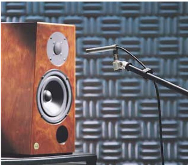
Test assemblies for electroacoustic converters frequently consist of microphones and loudspeakers, whose frequency response must be compensated. The equalizer function of the R&S UPL furnishes tailor-made solutions for such tests. Comprehensive test routines can be implemented with the aid of the universal sequence controller.
